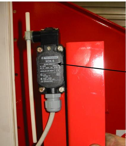
Limit switch contact to be put on the machine (mechanical stops to be fixed on the rail)
